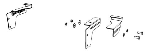
( **B** ) Secure the adjustable Wing assemblies from Step 2A to the Drawer System using four M6 x 16 Hex Bolts, four M6 Spring Washers and four M6 x 19 Flat Washers (Items 10, 14, 11) as shown.
