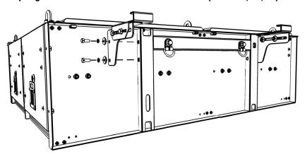
( C ) Fit the Left and the Right Front Faces (Item 21) to the Drawer System using the four M5 x 12 Button Head Bolts , four M5 Flat Washers and four M5 Nyloc Nuts (Items 18, 19, 29) as shown.
