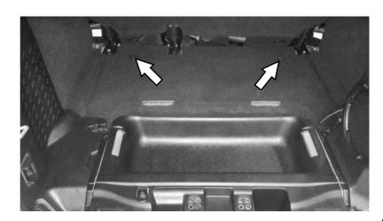
Working at the rear of the Drawer System, remove the top M6 Hex Bolt on both the left and right hand side of the Drawer. Secure a D-ring (Item 4) to each corner using a M6 x 20 Hex Bolt, M6 Spring Washer and M6 Spring Washer (Items 5, 6, 7) as shown.
