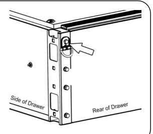
( **F** ) Remove the Cage Nuts from the left side, right side and rear of the Drawer as indicated by the arrows. When removing the rear cage nuts, lie the Drawer System on its side and open the Drawer to gain access.
