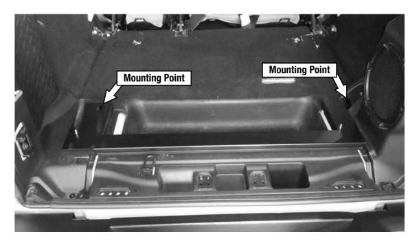
( B ) Place the Drawer System into the vehicle. The front square cutouts in the base of the Drawer sit over the studs in the Mounting Plate as shown. Secure the Drawer to the vehicle using two M6 Nyloc Nuts and two M6 x 19 Flat Washers (Items 15, 16). Place a M6 Nut Cap (Item 12) over each of the Nyloc Nuts.
