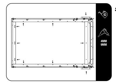
Make sure you have closed the load bed tail gate to ensure that it does not make contact with the frame. Once you are satisfied with the positioning of the frame, mark the position of all the mounting points as indicated by the arrows onto the load bed.
