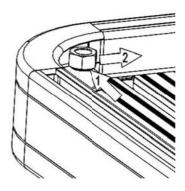
( **B** ) Position the Bottle Opener above the Nyloc Nut, lining up the hole in the top of the Bottle Opener with the Nyloc Nut. Fasten the Bottle Opener to the rack using the Button Head Bolt and Flat Washer supplied.
