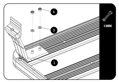
Loosely fit the Legs (Item 1) using M8 x 16 x 1.6SS Flat Washers and M8 Nyloc Nuts (Items 3 & 4).
