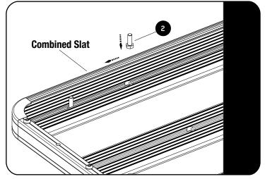
Slide two M8 x 25 Hex Bolts (Item 2) into the Slats machined slots.
