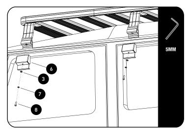
Secure the Gutter Clamps (Item 6) using M8 x 30 Button Heads, M8 SS Spring Washers and M8 x 16 x 1.6SS Flat Washers (Items 3, 7 & 8).
