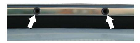
(B) Loosely fasten the Foot Rails (Item 1) to the vehicle's as shown below using the M6 x20 Button Head Bolts M6 Spring Washers and M6 Flat Washers (Items 5, 6, 7) supplied. The Product Sticker on the Foot Rail, must go to the rear and face the outside of the vehicle.
