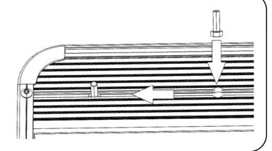
(B) With your Rack still upside down from Step 3A, slide a M8x20 Hex Bolt (Item 2) into the ends of each Slat. Place a M8 Flat Washer and M8 Nyloc Nut (Items 3 & 4) onto each bolt. Hand tighten the Nyloc Nuts until they begin to take on the nylon.
