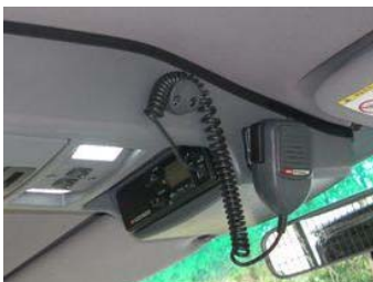
Install microphone clip on slight angle (same as console)
