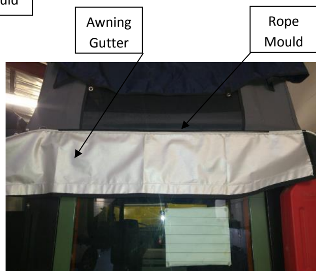
Figure 12: Gutter Installed into Rope Mould
