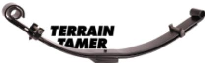
**LAMES PARABOLIQUES DE SUSPENSION AVANT
